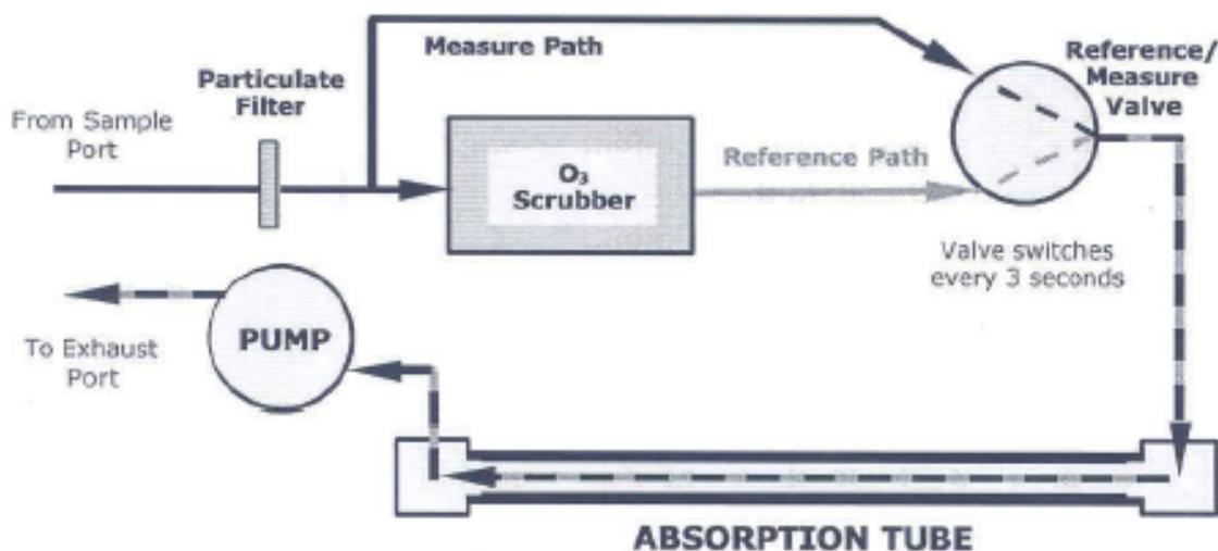
Figure 1. Reference cycle/Gas measurement.
