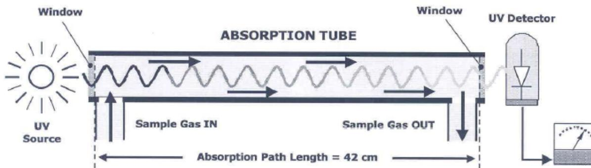
Figure 2. Detail of the O<sub>3</sub> absorption.
